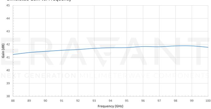
**Simulated Gain vs. Frequency**
