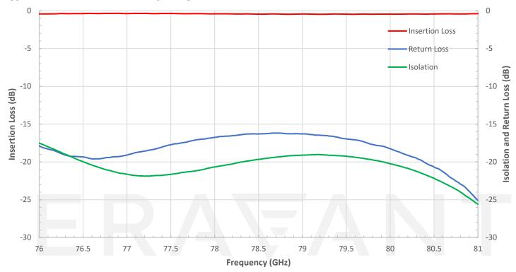
Note: The insertion loss, isolation and return loss between other ports, such as port 2 to port 3, port 3 to port 1 are similar to above given plots.
